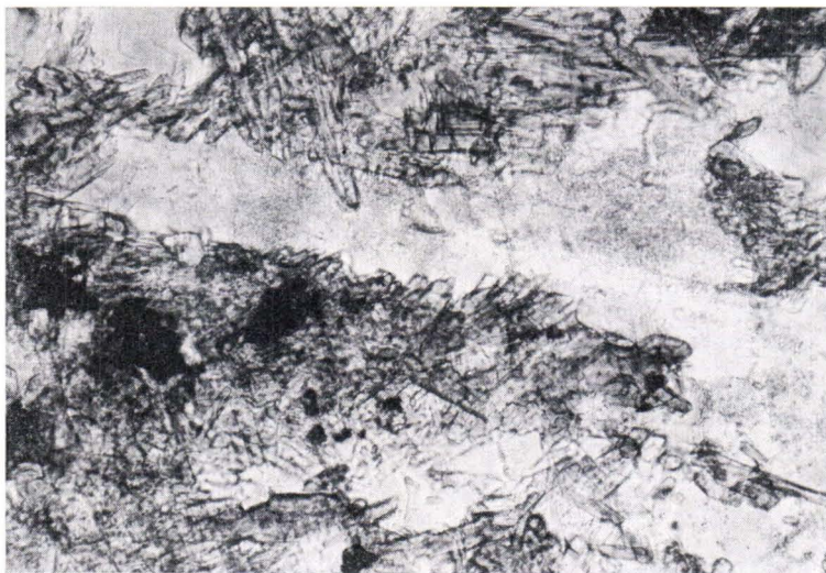
Fig. 22. Small prisms of hornblende forming a dense network between plagioclase borders. Note how the hornblende has grown into the pigmented and brown-coloured plagioclase (no. 136).
