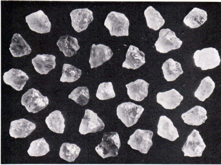
Fig. 34. Photograph of quartz grains. Sample No. 17. The 1—1.2 mm fraction. Very angular ( \alpha_1 ), angular ( \alpha_2 ) and subangular ( \beta_1 ) classes. Photo: E. Halme.
