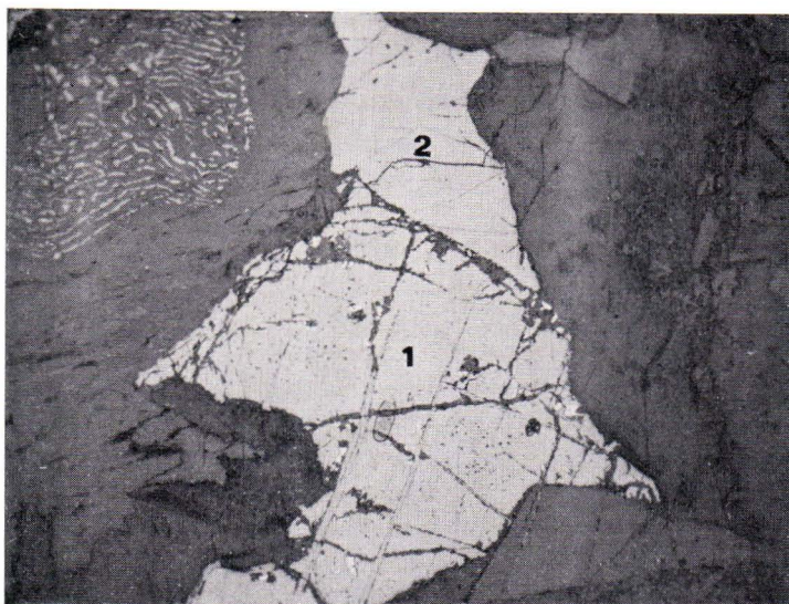
Fig. 10. Ilmeno-magnetite (1), consisting of ferrian ilmenite lamellae parallel to \{111\} in a titaniferous magnetite host, and forming a composite grain with coarse, irregular ferrian ilmenite (2). The ilmeno-magnetite also contains small inclusions of chalcopyrite (white). On the left is seen an intergrowth of orthopyroxene and ilmenite. Lower zone, sample 2. Magn. 70X.
