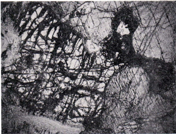
Fig. 6. An entirely anhedral grain of partly serpentinized olivine resulting from pronounced adcumulus growth. (Sample 3). Magn. 18X. Without analyzer.
