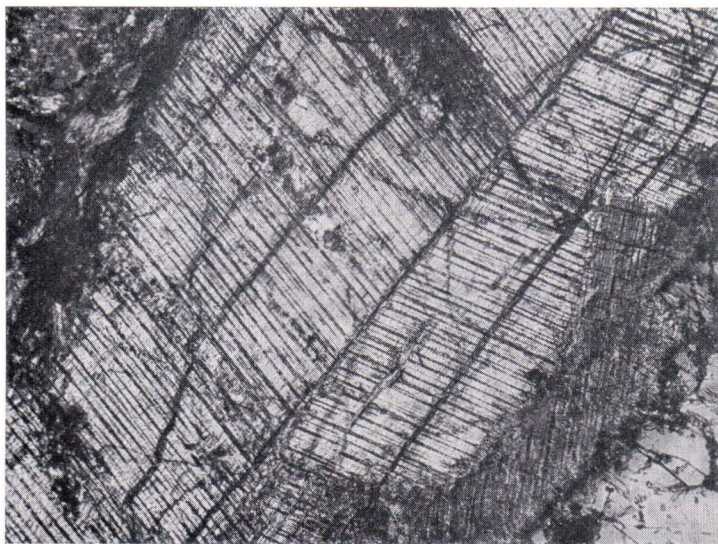
Fig. 9. Exsolution lamellae of pigeonite in twinned augite parallel to (001) plane of augite host forming the herringbone pattern. Middle zone sample 11. Magn. 60X. Crossed nicols.
