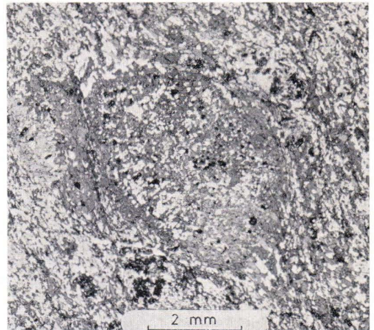
Fig. 10. A vesicle within an intermediate volcanic rock filled with dark hornblende, quartz and opaque minerals. One nicol. Virkamäki, P 109/MH/65.
