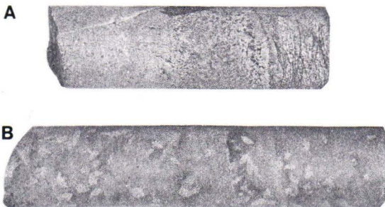
Fig. 61. Drill cores from rocks of the Kiihtelysvaara Turbidite Suite. A) Graded-bedded quartzite from the lower part of the Turbidite conglomerate—quartzite Formation (drill core No. R311/4241/80.50). B) Mica schist with staurolite porphyroblasts from the lower part of the Mica schist Formation (drill core No. R311/4241/41.75). Both samples from the Viistola area at Kiihtelysvaara. Drill cores about 32 mm in diameter. Photo by E. Halme.
