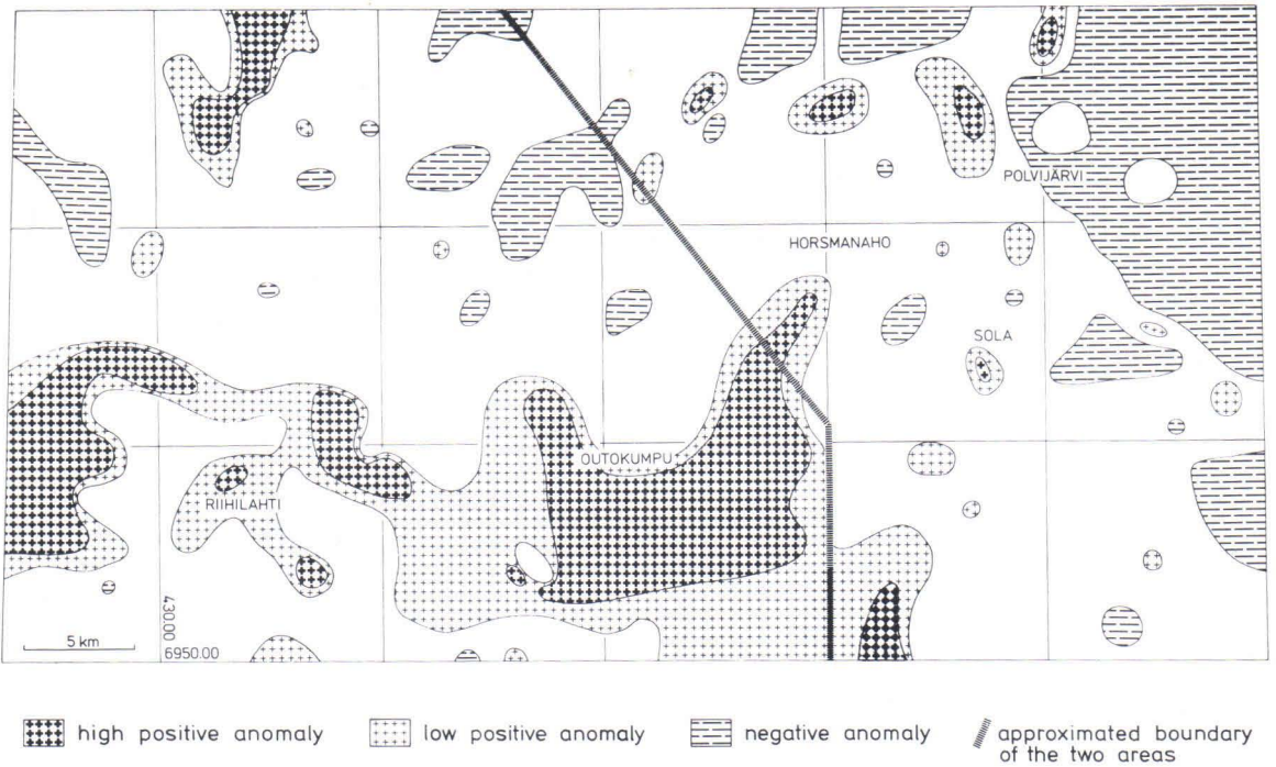
Fig. 30. The nickel content of the < 0.06 mm till fraction on the surface (1.0—1.5 m) of the till blanket in the Outokumpu—Polvijärvi area. The anomaly thresholds are the same in the whole area. See also Tables 1 and 2.
