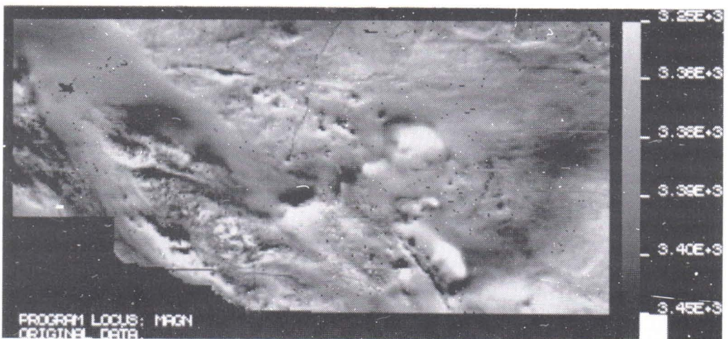
Fig. 3. The greytone image map prepared from aeromagnetic data by removing data points with mean value of the total field. The points removed appear as black dots.
