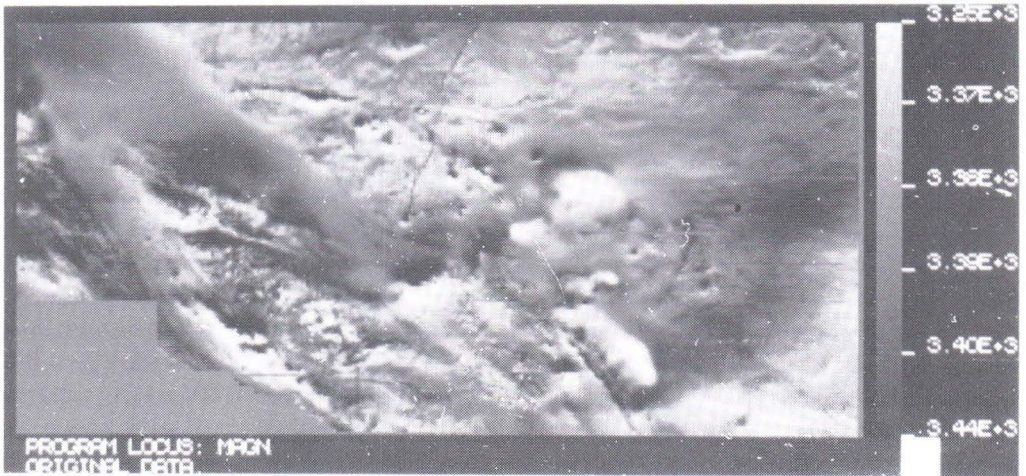
Fig. 2. The greytone magnetic map prepared from digitized data. The light tone indicates low intensity magnetic anomalies and the dark tone corresponds to high intensity magnetic field.
