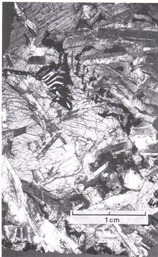
Fig. 3. Microphotograph of olivine diabase from Märket with typical skeletal magnetite and ophitic texture. + nicols. Photo Erkki Halme.
