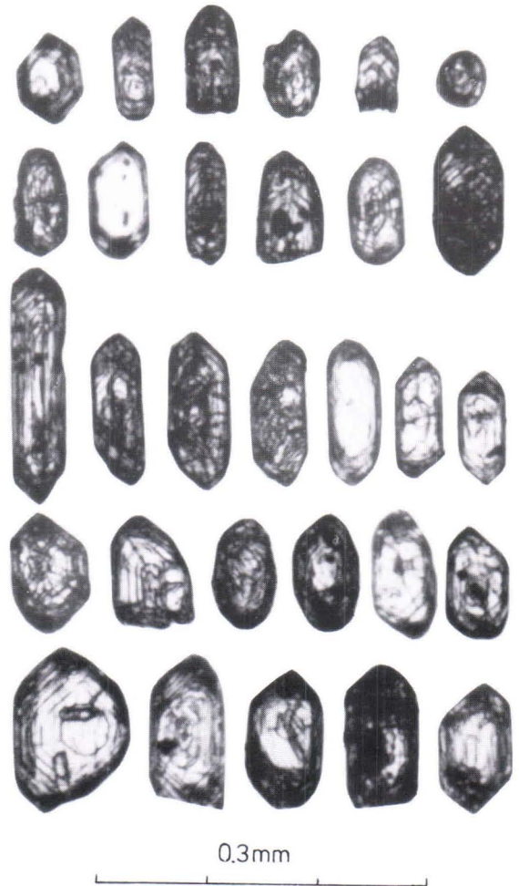
Fig. 60. Microphotographs of zircon crystals from granodiorite A563-Algersö. Zonal growth on a growth nucleus is present in all crystals, although the habit varies markedly.
