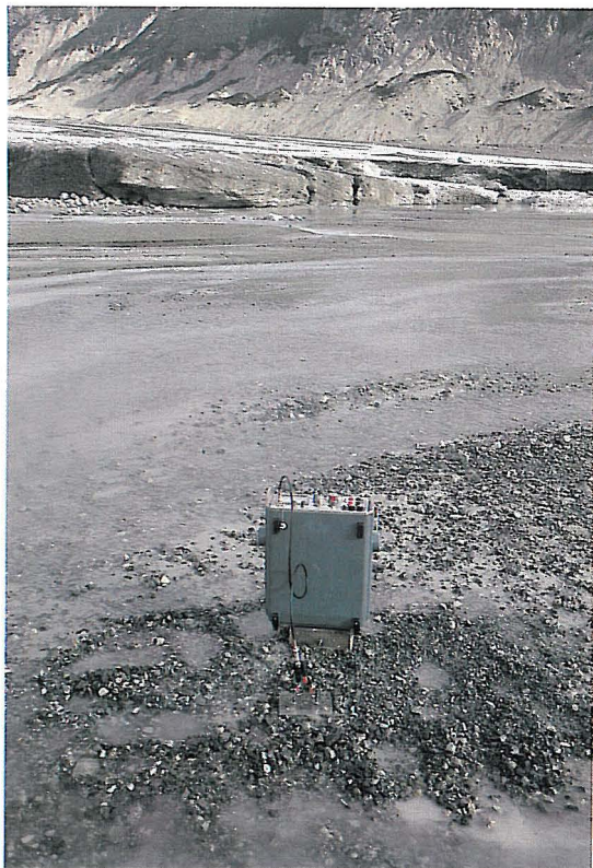
Fig. 32. An in situ TDR determination of saturated outwash deposits ( \epsilon_r = 24.9 ; \sigma = 0.0028 S/m; \sigma_{\text{water}} = 0.0075 S/m) close to the margin of the Burroughs Glacier, southeast Alaska. Photo R. Sutinen 1988.
