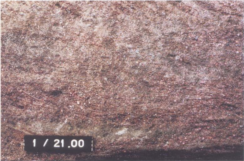
Fig. 8. Poorly sorted, coarse grained sandstone of St_1 -facies. Harjavalta, profile 1A, 21 m. The length of the tag is 16 cm.
