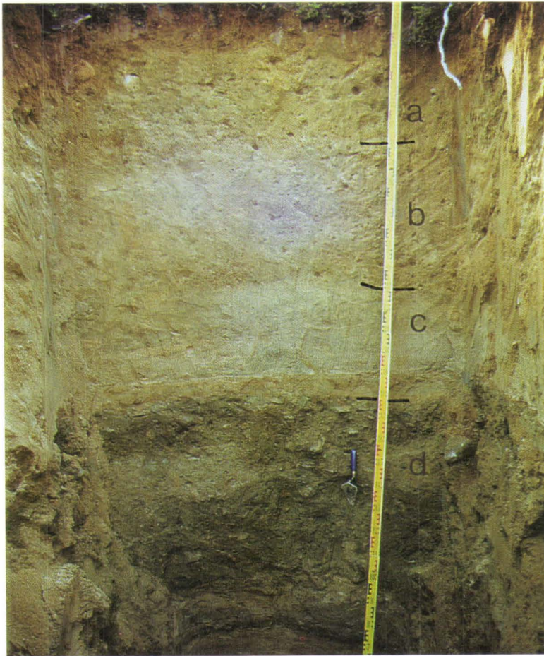
Fig. 23. The youngest till unit (a), the 'Old Northern' till unit (b), a sand unit belonging to a NW-SE-oriented esker (c), and the oldest till unit (d) in the wall of an excavator pit at Suomurinivat.
