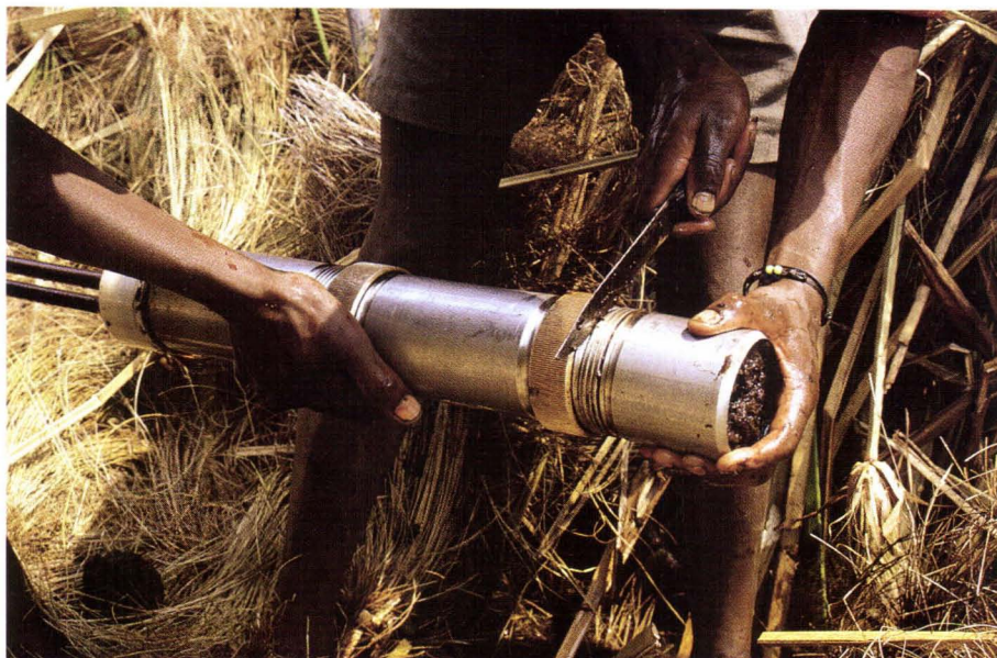
Fig. 7. Samples for laboratory analyses were taken with a volumetric piston sampler. Volumetric samples are necessary for calculation of the dry bulk density and the rate of peat accumulation.
