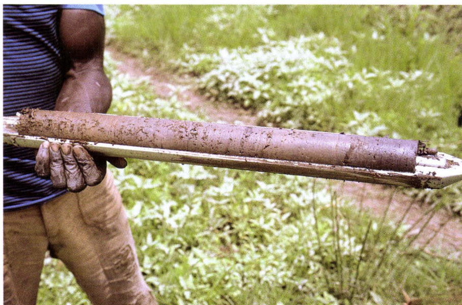
Fig. 8. Samples were taken with a Russian-type peat sampler for use in both field and laboratory determinations.
