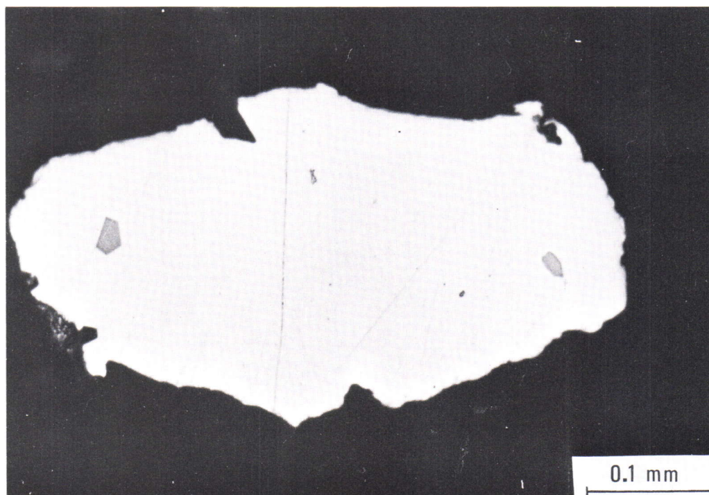
Fig. 13. A gold grain from Hangasoja with arsenopyrite inclusions. Optical micrograph.
