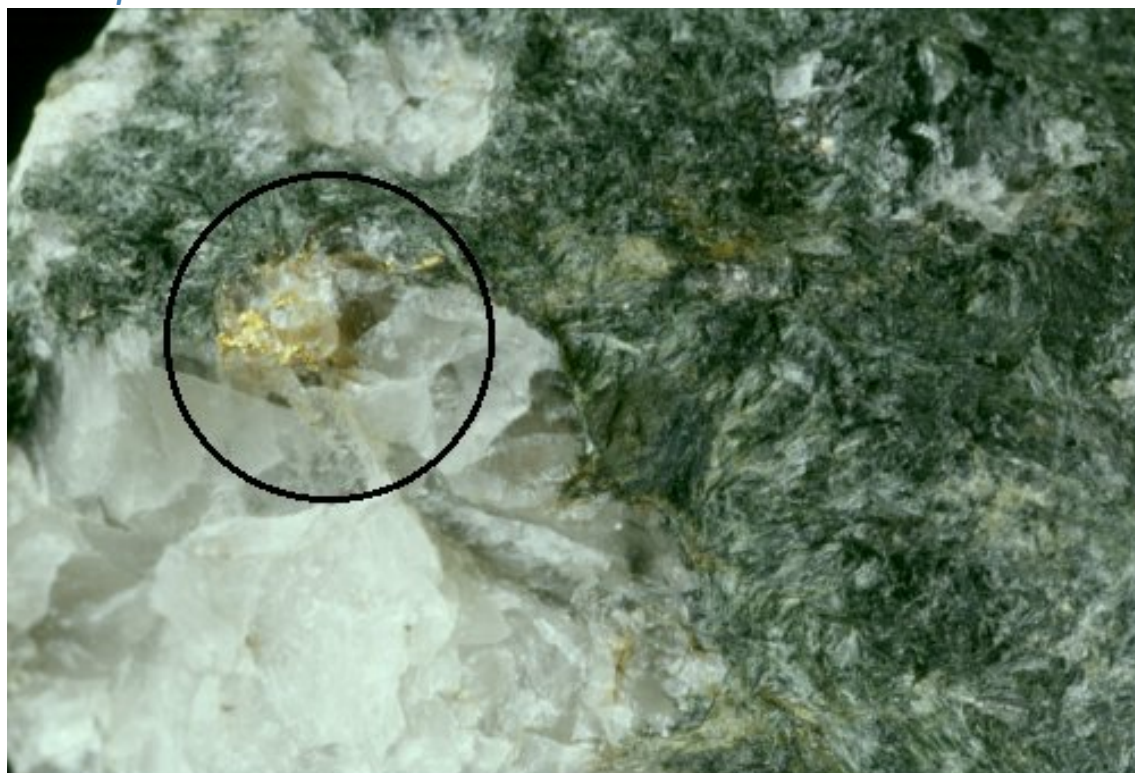
Gold (encircled) at the contact between a quartz vein and the komatiitic host rock in high-grade ore at Pahtavaara, Sodankylä. The mineral assemblage of the altered komatiite is here dominated by tremolite with minor biotite, dolomite and quartz. Field of view is approx. 5 cm. Photo Jari Väättäinen.
