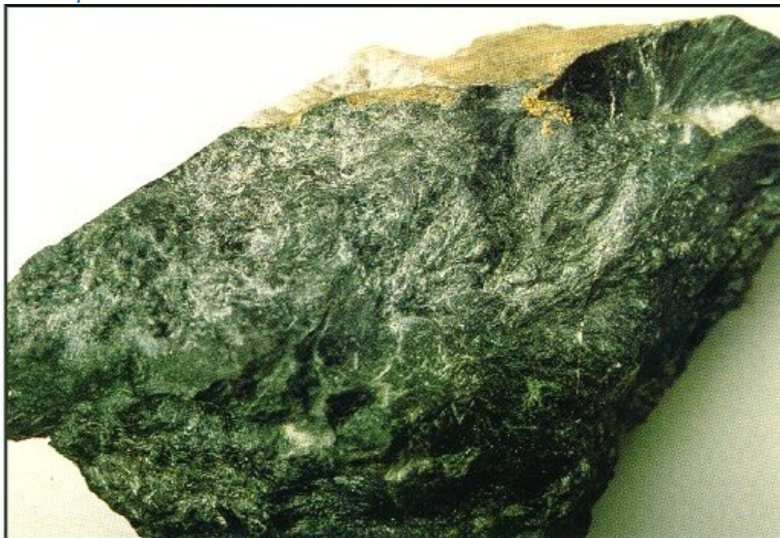
Visible gold (yellow) in contact zone between a quartz-barite vein (white) and coarse-grained amphibole rock (green). Exploration Trench 5, high-grade ore. Field of view is 10 cm in width. (from Korkiakoski 1992)
