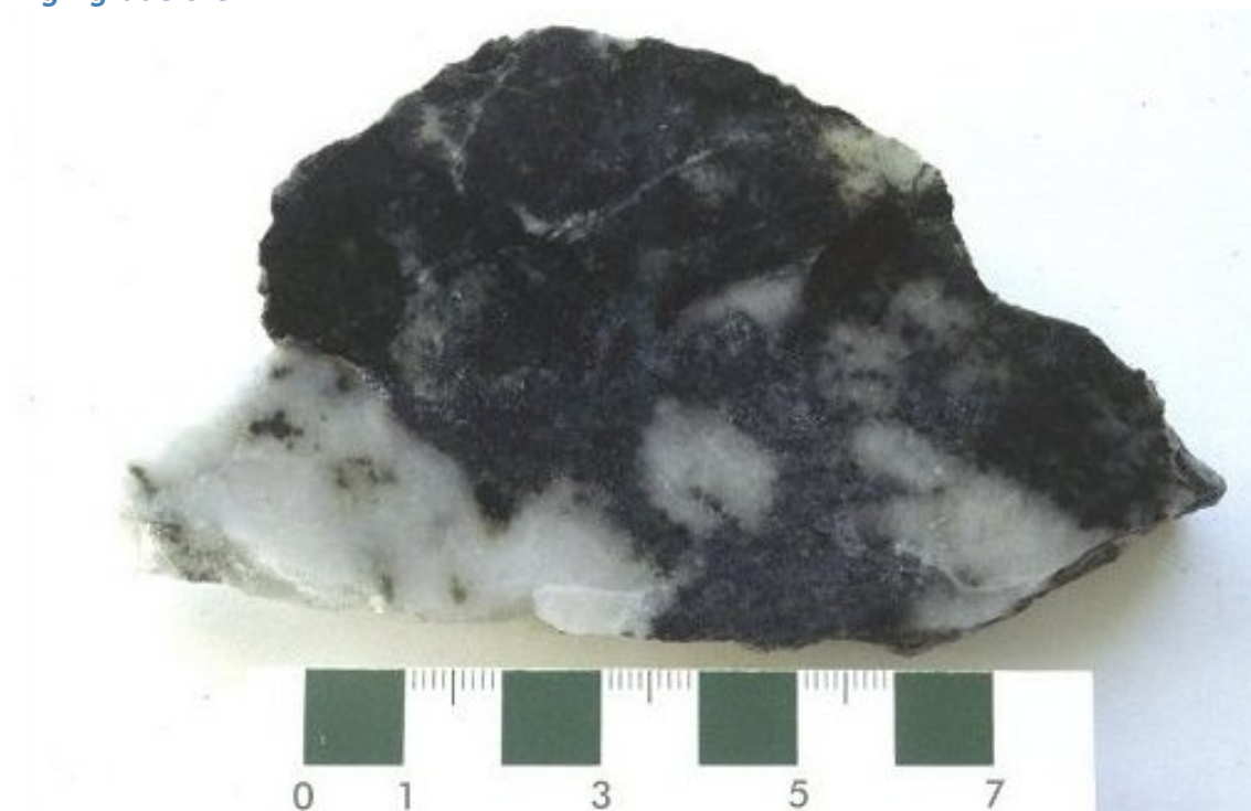
Pahtavaara, Sodankylä. High-grade ore (several tens of ppm Au). White quartz-baryte vein material, and dark green (tremolite-rich) and black (biotite-rich) altered host rock. Scale is in cm.
