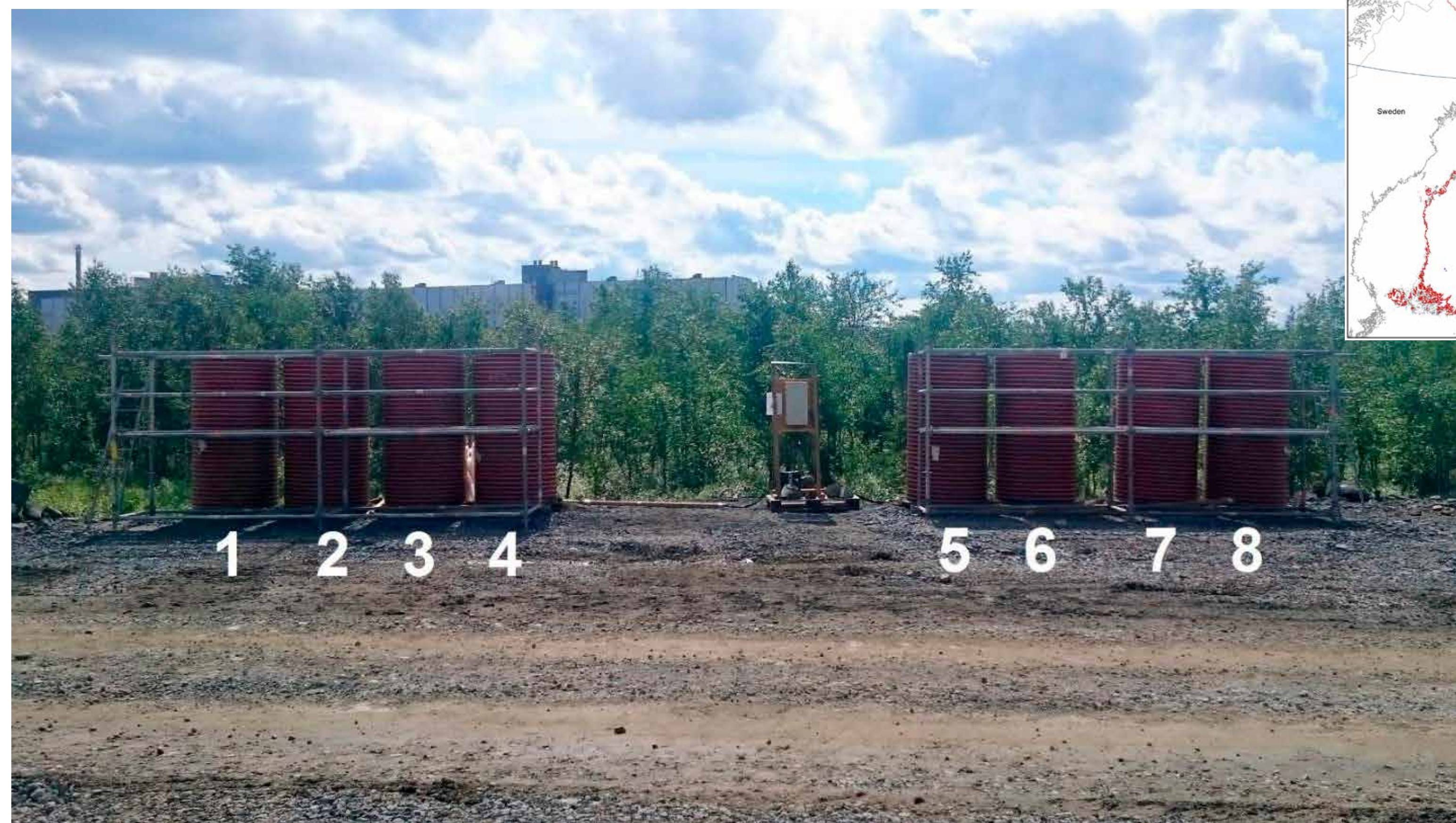
Fig 1. Eight waste rock lysimeters and the data logger unit at the Kevitsa mine, Finland. Lysimeters are 1 m diameter and 2 m high plastic cylinders with sensors for moisture, temperature, electric conductivity and oxygen.
