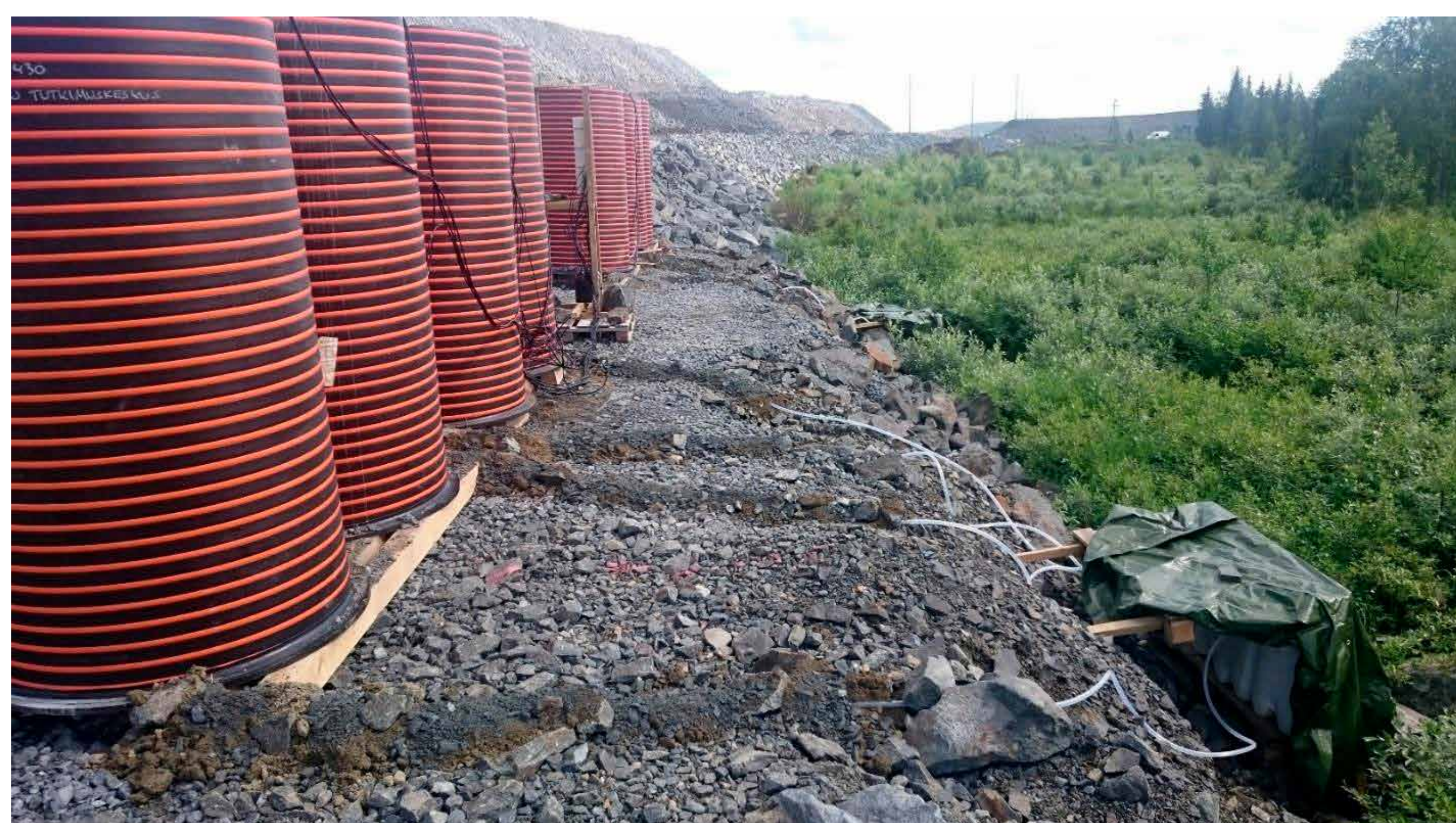
Fig 3. Drainage waters are conducted to canisters below the lysimeters.
