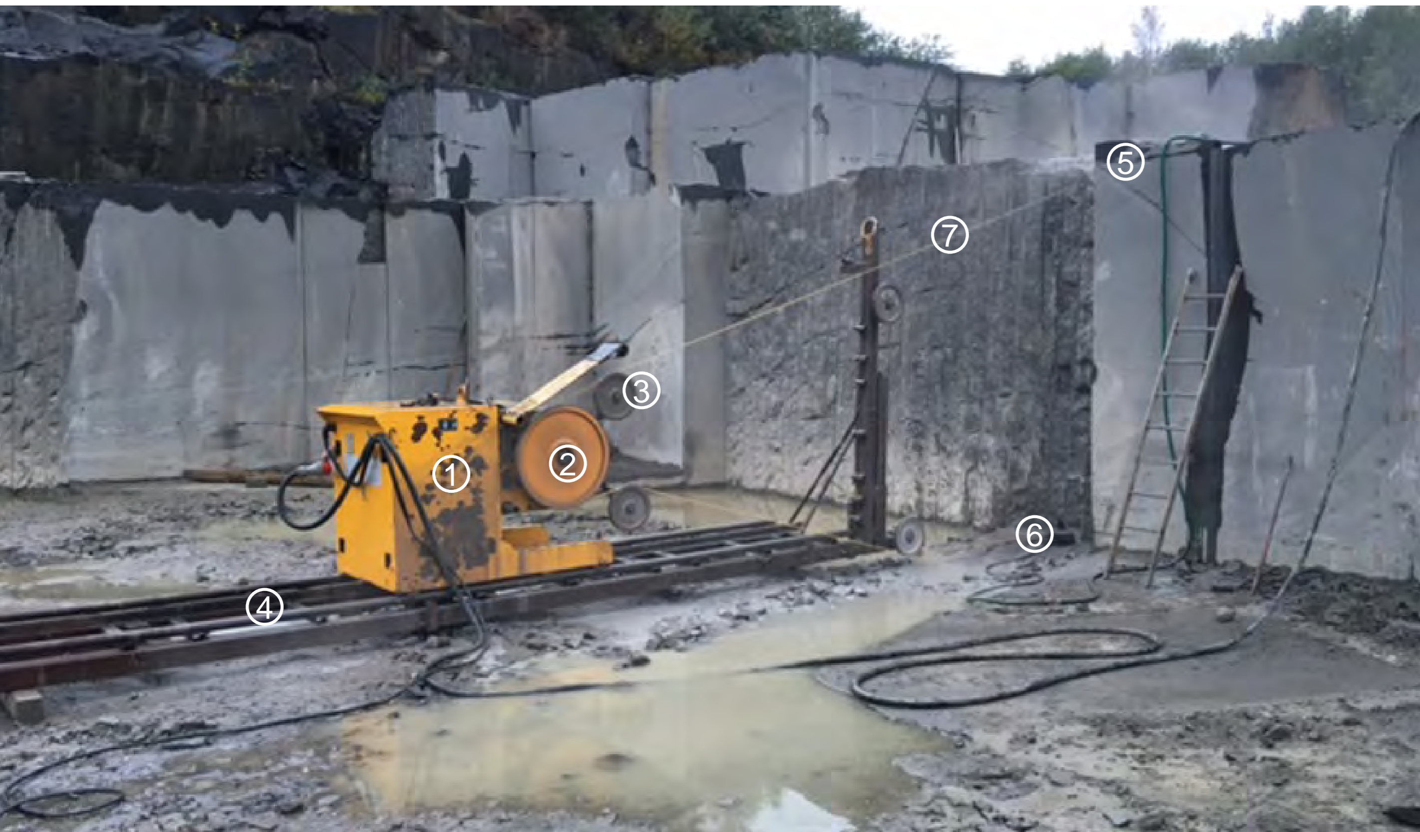
Figure 1. A wire cutting test of gabbro at Oulainen quarry in western Finland. 1. saw unit, 2. flywheel, 3. pulley, 4. tracks, 5. flushing water, 6. access holes 2. for the wire, 7. diamond wire loop.
