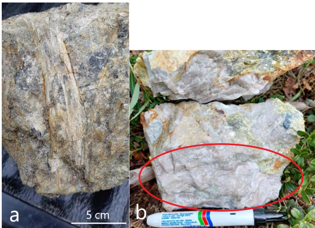
Fig. 16. LCT pegmatites found from the study area in Lapua–Kuortane. a) A spodumene-bearing boulder from Kurjenneva. b) Montebbrasite–amblygonite (encircled) from Pikkalantausta.
