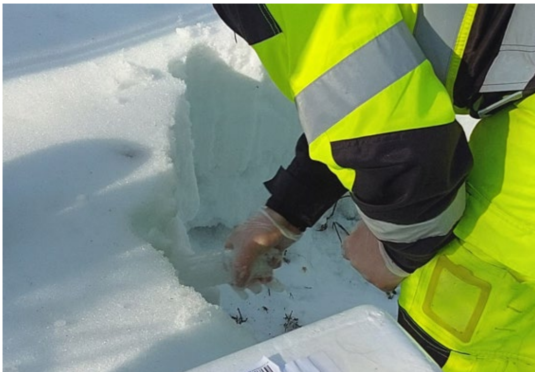
Fig. 3. A snow sample being taken into an acrylic tube. Kaustinen, March 2022. Photo: S. Leinonen.
