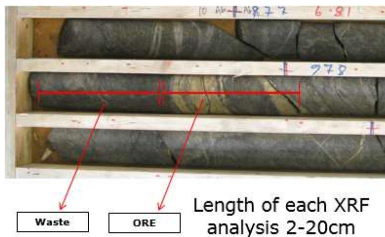
Figure 137. scanning analysis of drill cores in short length averages (2-20cm range) (Ilpo Auranen IMA)
