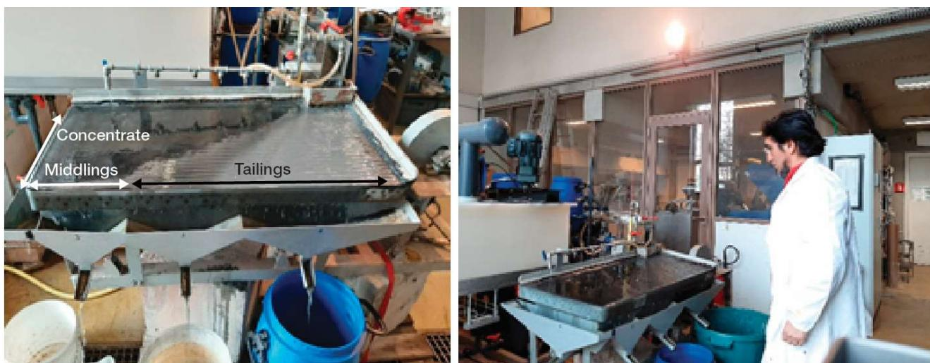
Figure 58. Photographs of the shaking table test work
