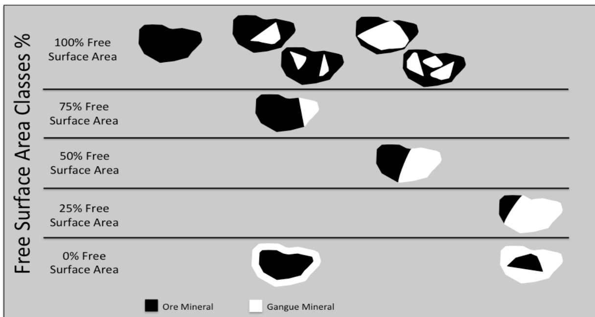
Figure 29. Different rock textures, each would have a different process recovery (Source and copyright: Cropp 2013)
