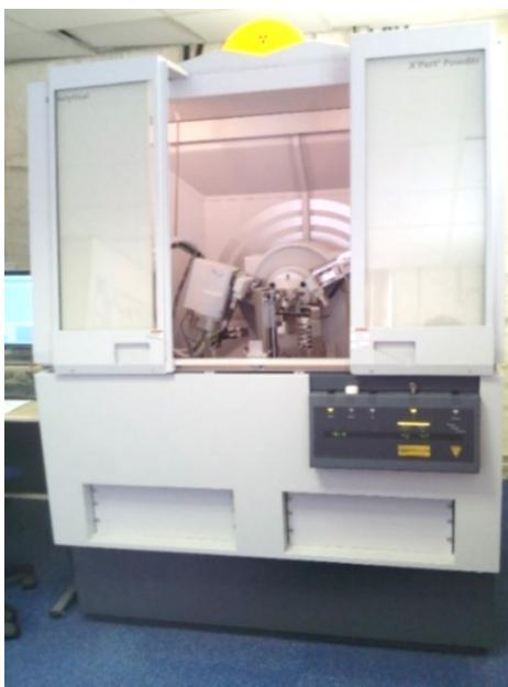
Figure 11. The PANalytical X'Pert3 diffractometer diffractometer using a CuK $\alpha$  radiation at 40 kV and 40 mA
