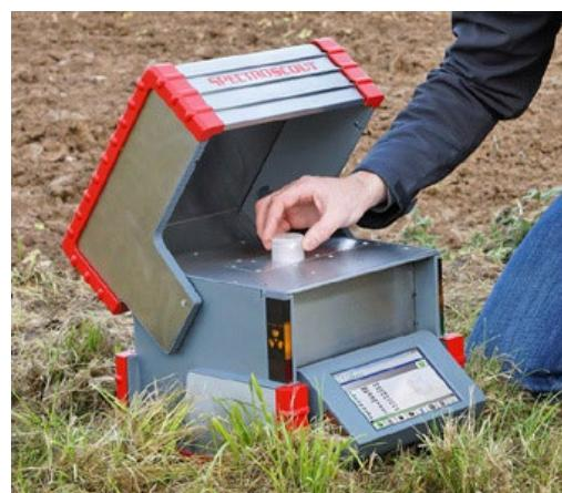
Figure 41. The portable benchtop Spectroscout (by Spectro) ED-XRF spectrometer
