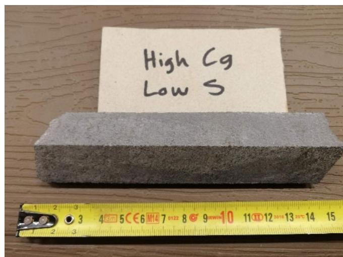
Figure 20. Aitolampi ore type, High Carbon, Low Sulfur – QA2
