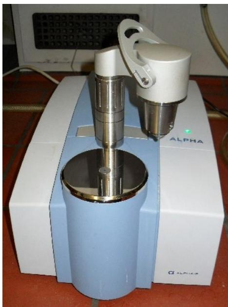
Figure 56. Bruker Alpha instrument with an ATR stage and a M-IR range of 4000-400 1/cm
