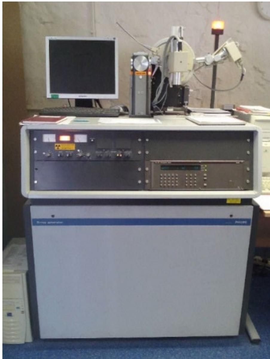
Figure 40. Philips PW1730 Generator using CuK $\alpha$  radiation at 40 kV and 40 mA.
