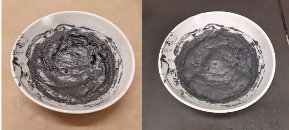
Figure 5. Graphite concentrate and sodium hydroxide before (left) and after (right) alkaline roasting at 150–350 °C in a chamber furnace in GTK Mintec Laboratory in Outokumpu.
