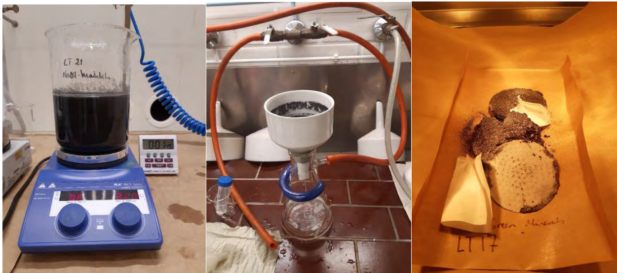
Figure 6. Water wash of alkaline roasted graphite concentrate in the beaker (left). Filtration with the vacuum filter (middle). Final graphite concentrate (right).
