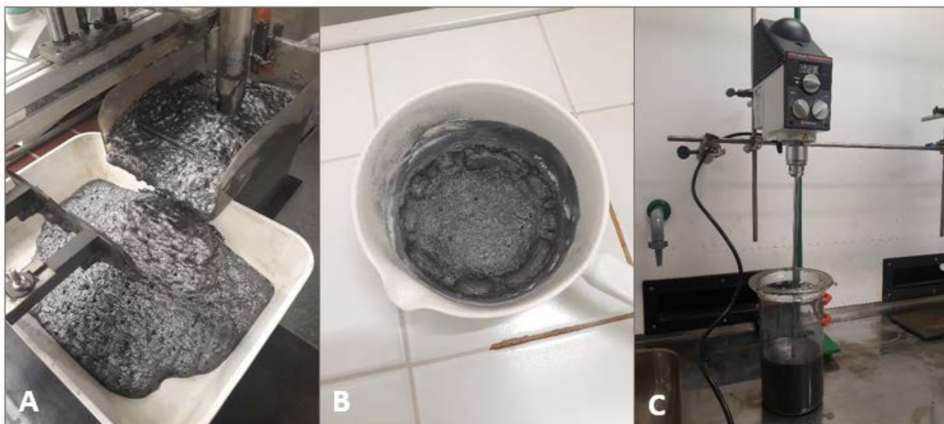
Figure 1: Graphite concentrate production procedures. A: Graphite concentration by flotation. B: Graphite concentrate after alkaline roasting. C: Acid leaching procedure.
