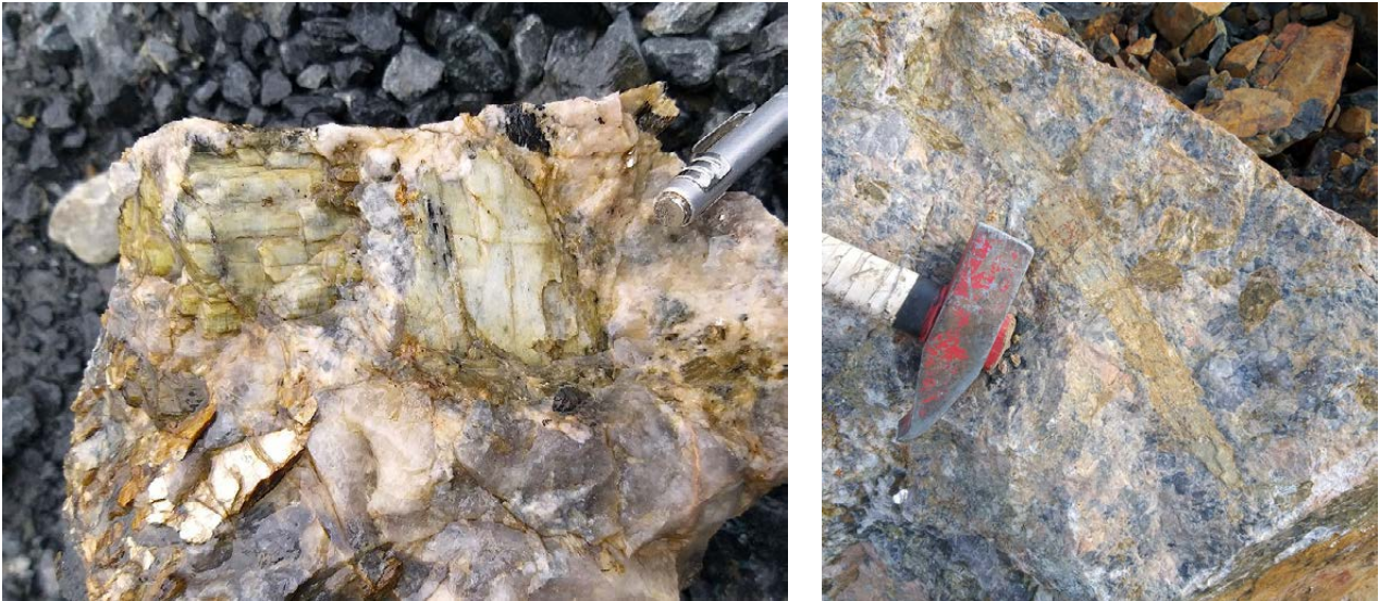
Fig. 20. Left: Light green spodumenes in a rock sample. Right: the southern dyke shows up to 30-cm-long beige-coloured spodumenes (hammer head ca. 10 cm in size).
