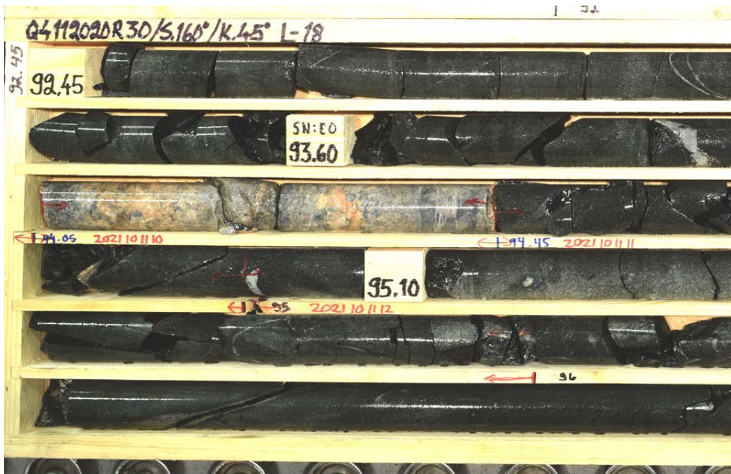
Fig. 25. A 0.40 m pegmatite dyke in drillhole R30, 94.05–94.45 m, wet core.
