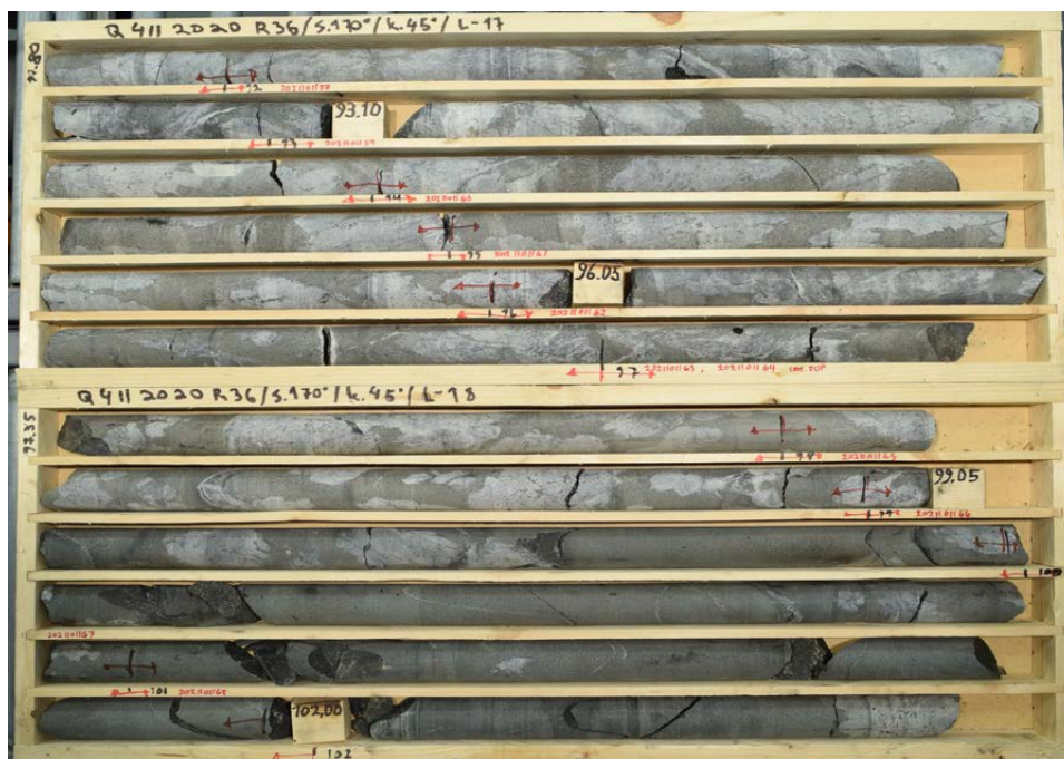
Fig. 26. Drill core of R36, showing the latter part of the possible pegmatite fluid-altered section 86.50–99.50 m. The host rock is amphibolite.
