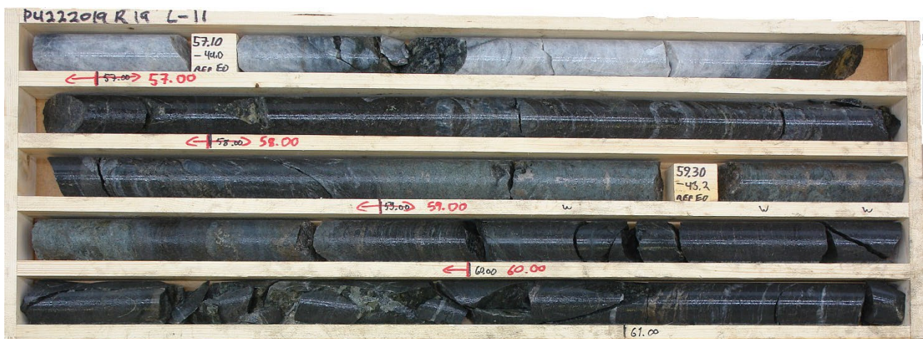
Fig. 4. Kedonkangas drill hole R19 with silicified black schists and volcanic rocks. The section 59 – 60 m contains nearly 0.2 % W.
