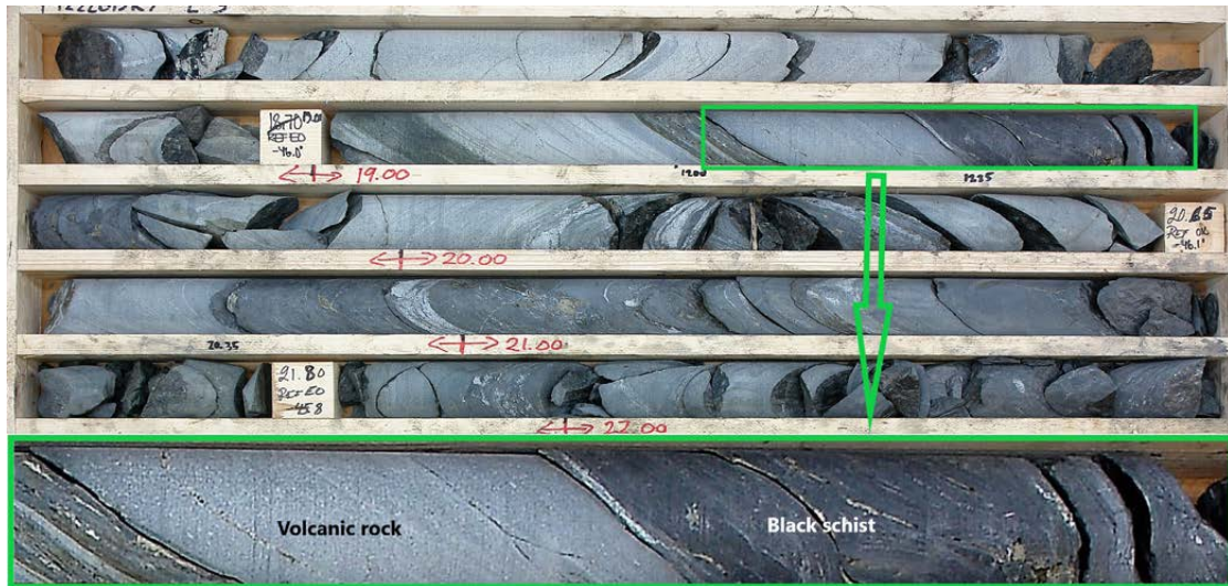
Fig. 9. Drill core box from drill hole R7. Black schists are often intertwined with volcanic tuff layers.
