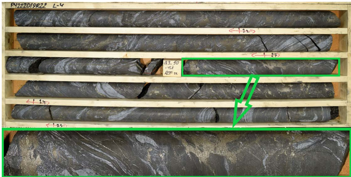
Fig. 18. A part of Emas black schist section 16–32 m from drill hole R22 with an average flake graphite content of 7.2%. The present sulphides are dominated by pyrrhotite and pyrite.
