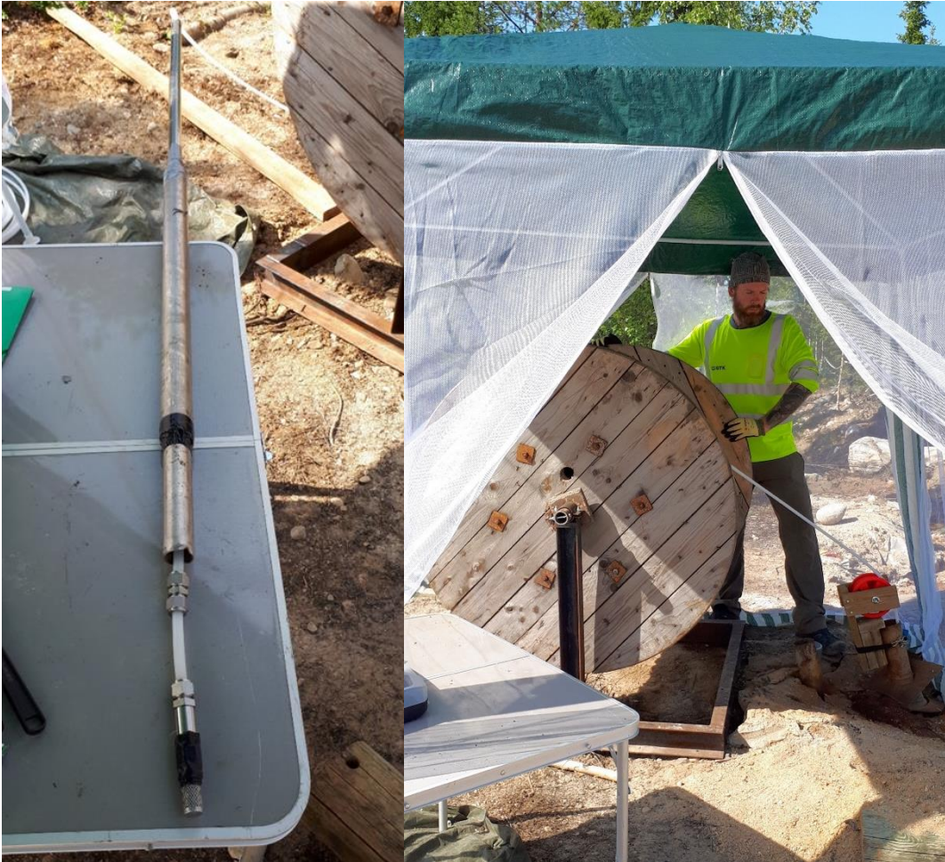
Figure 441. The head of the tube sampler (left). Lowering the tube into the drillhole (right).
