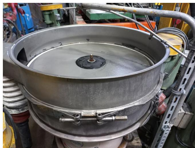
Figure 1. The graphite concentrate was sieved for the spheroidization tests using a Sweco vibration sieve.
