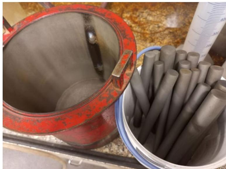
Figure 10. The primary grinding was performed with the mild steel rod mill.
