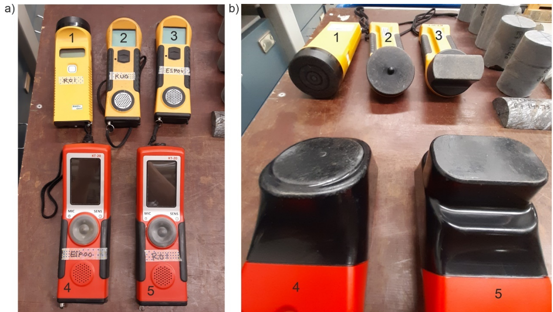
Figure 1. a) Kappameters' display and control panels, and b) sensorheads. 1 = KT-6 with a round sensor, 2 = KT-10 v2 with a pin sensor, 3 = KT-10 v2 with a rectangular sensor, 4 = KT-20 S/C with a round sensor, 5 = KT-20 S/C with a rectangular sensor.
