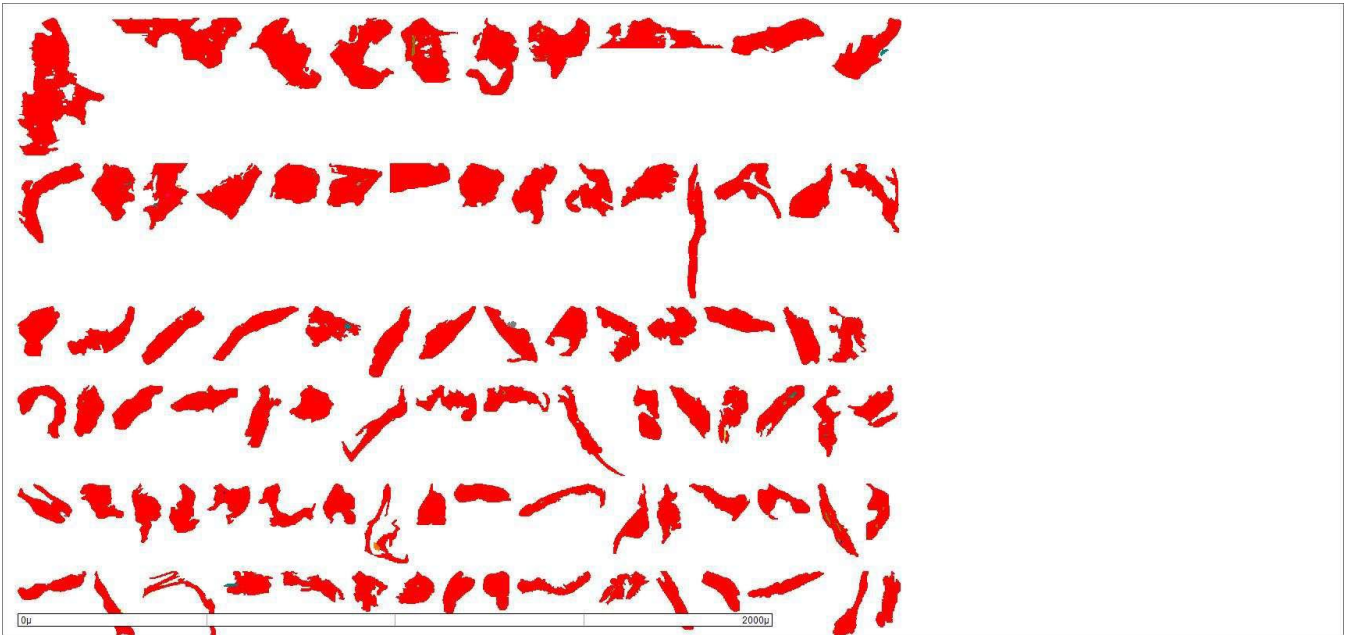
Figure 15. Particle images of graphite, Kämpysuo Blend 2, D50 50 μm.
