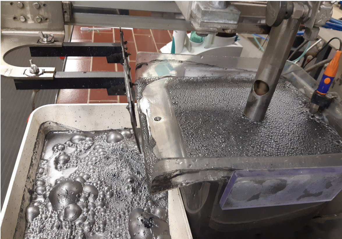
Figure 7. Graphite flotation, Luopioinen.
