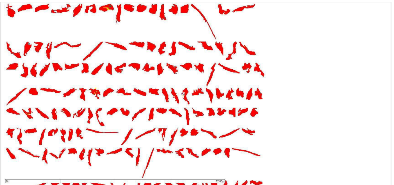
Figure 16. Particle images of graphite, Kämpysuo Blend 2, D50 50 μm.
