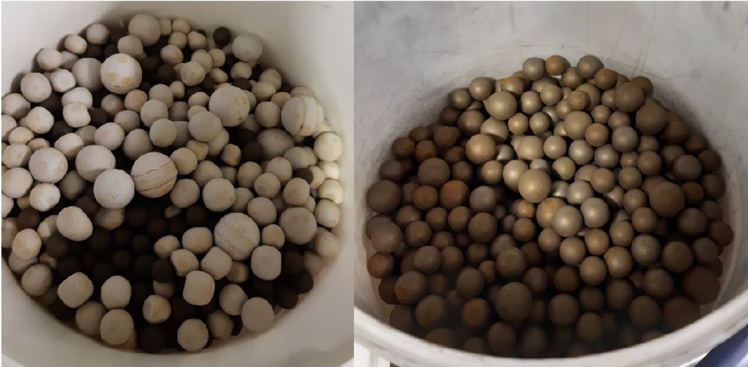
Figure 3. The used ball charges in graphite concentrate regrinding, combination of ceramic and steel balls on the left and steel balls on the right.
