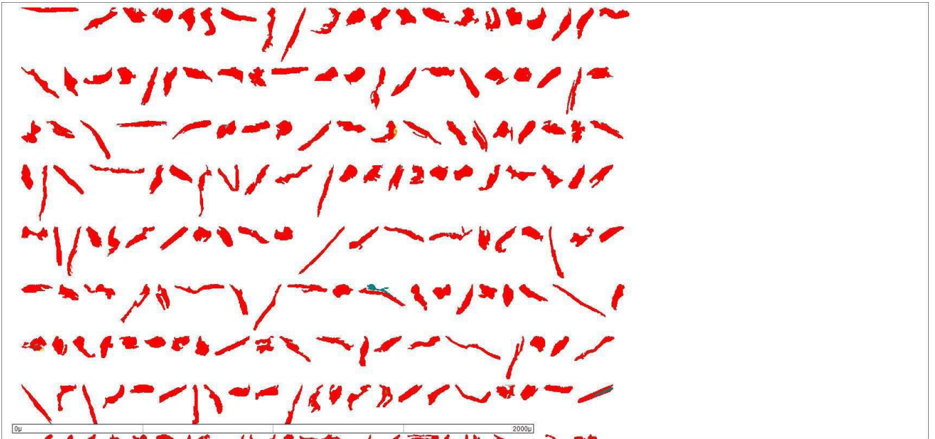
Figure 17. Particle images of graphite, Käpysuo Blend 2, D50 50 μm.
