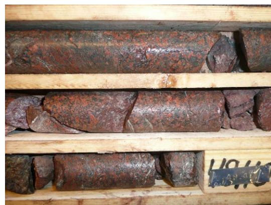
Figure 15. Pirttikoski drill core. Left: strongly deformed, fine-grained chlorite-carbonate schist, where the light bands are calcite and quartz (hole R306). Right: quartz and chlorite vein brecciated granitoid (hole R311).
