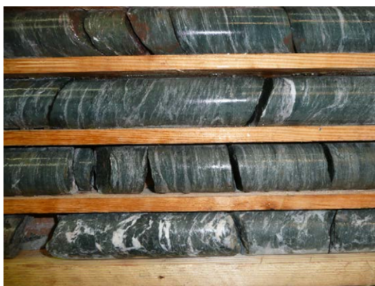
Figure 15. Pirttikoski drill core. Left: strongly deformed, fine-grained chlorite-carbonate schist, where the light bands are calcite and quartz (hole R306). Right: quartz and chlorite vein brecciated granitoid (hole R311).
