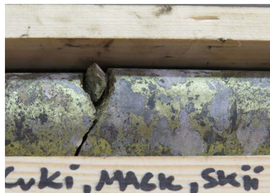
Figure 12. Left: Cu-REE mineralization in drill hole R39. Right: Cu mineralization in drill hole R33 from the eastern part of the Kotka study area.
