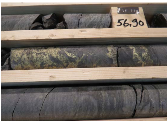
Figure 12. Left: Cu-REE mineralization in drill hole R39. Right: Cu mineralization in drill hole R33 from the eastern part of the Kotka study area.
